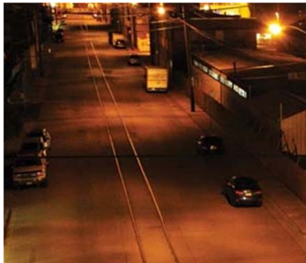
Before: 70W HPS Drop Glass Cobra Heads System Power - 95 Watts
