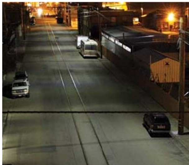
After: 40 LED Leotek Green Cobra System Power - 47 Watts
